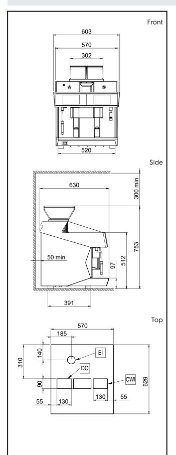
Electric Supply voltage: 602551 (TANGOST2SA) 400 V/3N ph/50 Hz Electrical power max.: 5.2 kW Plug type: Cable without plug Water: Cold water temperature (min/max): 5 / 60 °C **Key Information:** External dimensions, Width: 603 mm External dimensions, Depth: 629 mm External dimensions, Height: 833 mm Net weight: 130 kg 0.69 m<sup>3</sup> Shipping volume: Sustainability
